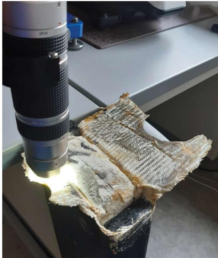
Fig. 4.1 – Analysis of fracture with a digital microscope.
