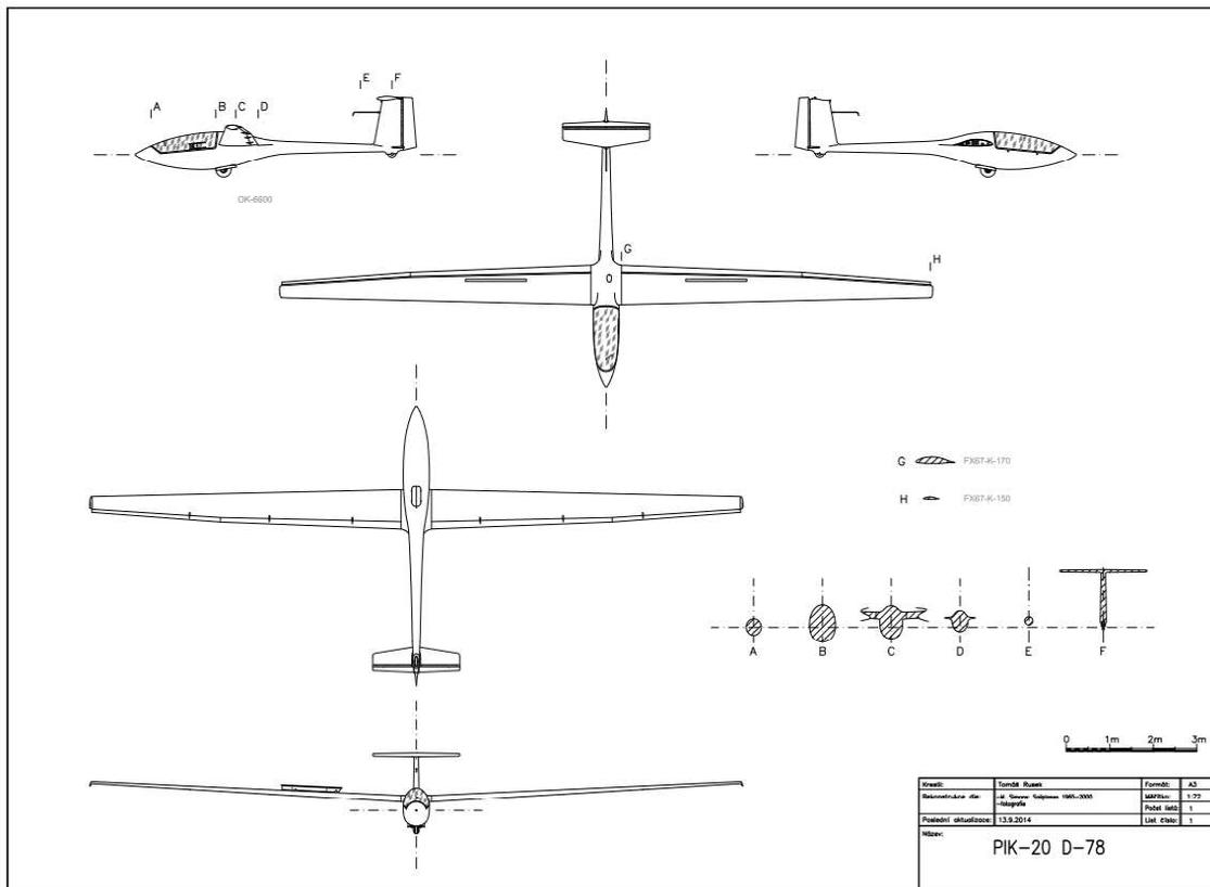
Fig. 2 – Scan of the technical drawing of the PIK-20D-78 glider
